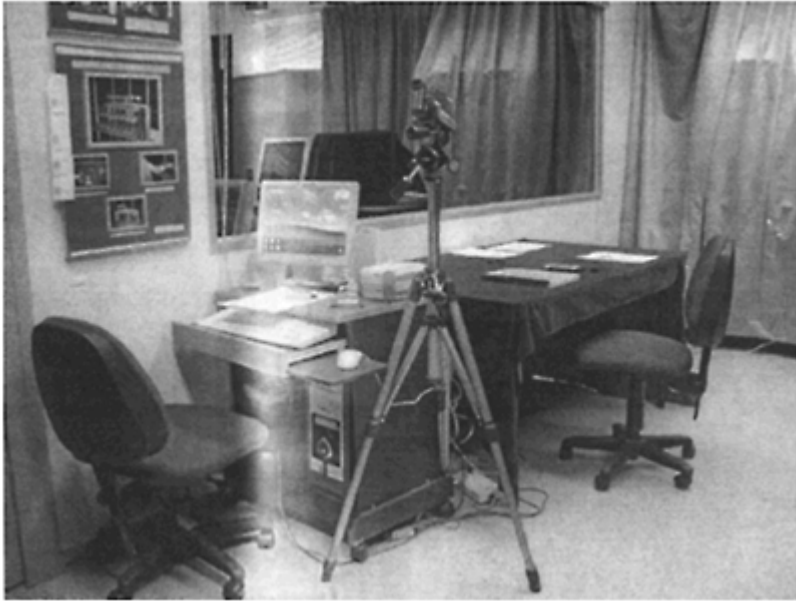
FIGURE 7.4 The usability lab at Nanyang Technological University. There are several video cameras hidden in the ceiling and behind the one-way mirror. User actions and voice comments are recorded on video recorders and analyzed. The user performance is evaluated and related to the interface design. Design improvements can then be suggested.
